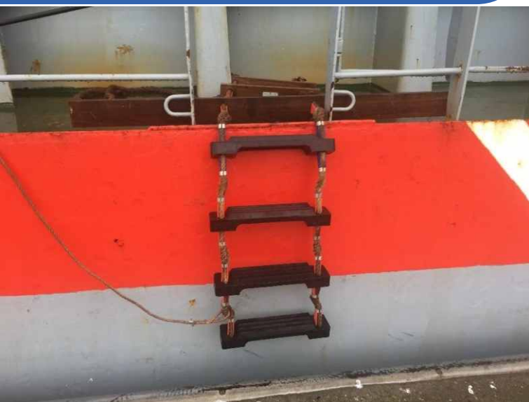
spreader used for secured the ladder behind a very thin piece of railing
