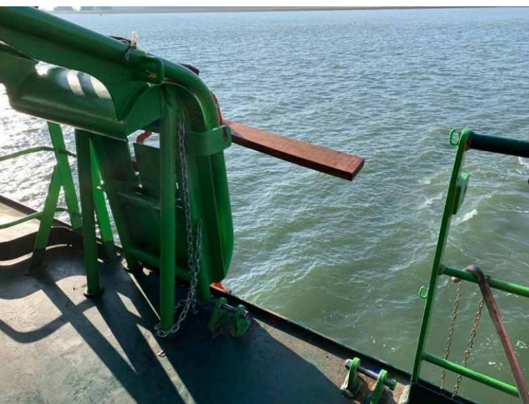
Non compliant (by design) pilot ladder winch reel, spreader obstructing entrance after the sideways dive.
