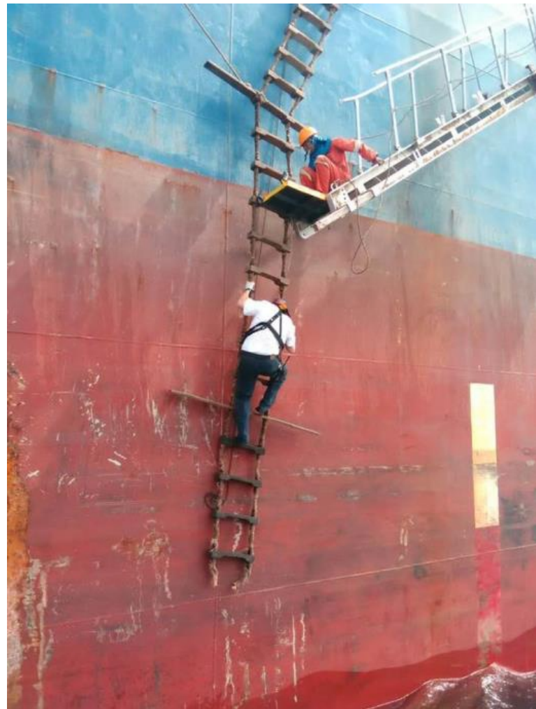
Non-compliant combination, (courtesy of #dangerousladders)
