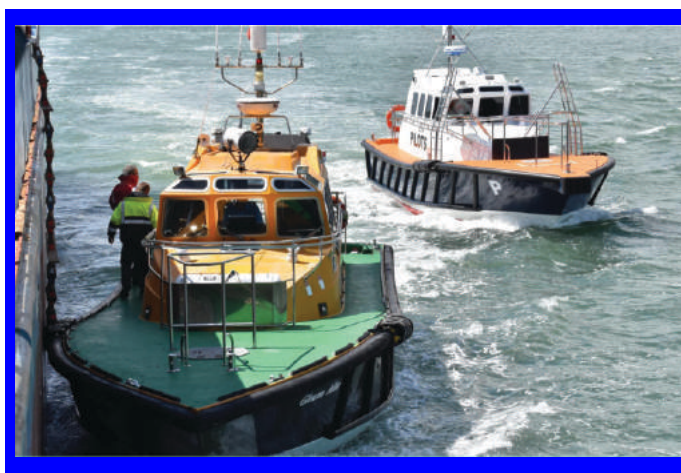
Above two Interceptor 42 Pilot boats for different ports and countries, one operating without a plot boarding ladder and one with. Below, one of our designs of pilot boarding ladder with the platform 1.1m above deck.
