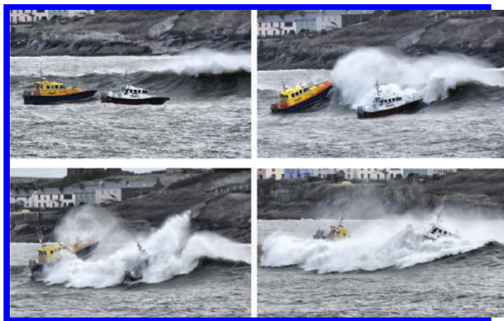
A Pilot 38 & 48 coxswain's having confidence in their boats seakeeping as they encounter large breaking seas during sea trials at the entrance to Cork Harbour, on the South coast of Ireland where Safehaven Marine are based.
