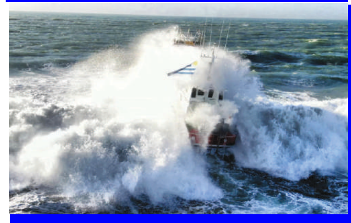
Above, a big breaking sea coming over the bow makes one appreciate the need for very strong windows. Below, a large lump of solid water running along the deck, a cubic meter of water weighing 1 ton travelling at 25kts.....
