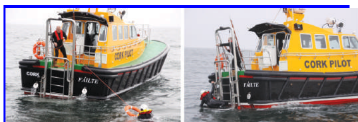
Above and below photos show the MOB recovery system in use with the casualty being drawn by life ring or boat hook to the platform, then being lifted to deck level.
