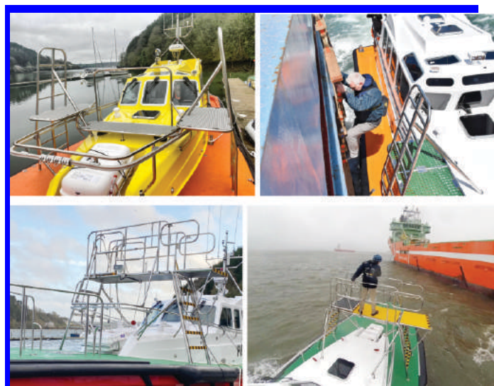
Above, another design with a platform 1.8m above deck with a hinged outer platform and handrail.
