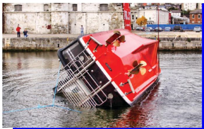
Above, an Interceptor 48 pilot undergoing a self-righting recovery test by being pulled over gradually to an inverted position by a crane to ensure she recovers to an upright condition simulating a capsize scenario.
