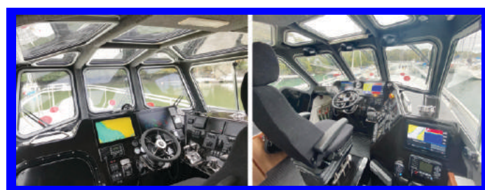
Above, the central helm position on our pilot boats gives the coxswain coxswain control of the vessel whether boarding from the port or St/bd side.
