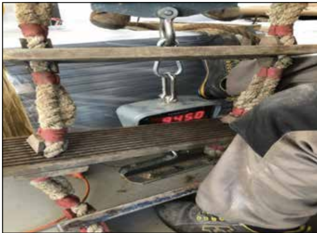
Durability test of the damaged pilot ladder at the premises of the producer.
