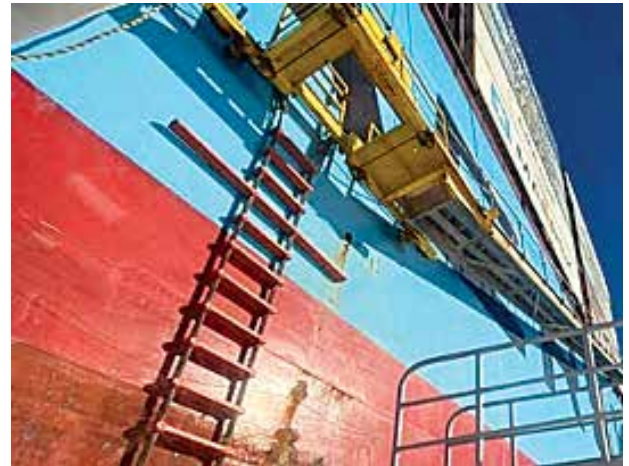
FIGURE 4 – LADDER NONCOMPLIANT. NOTE THAT TO CROSS THROUGH THE TRAPDOOR YOU'LL NEED MOUNTAIN-CLIMBING SKILLS...
