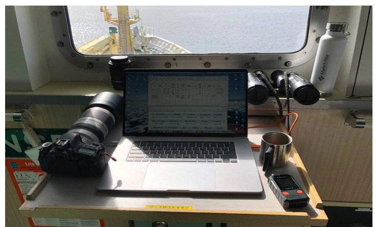
An Ice Navigators set up for working ice. The computer accesses ice charts and imagery, linked to the ships navigation sensors and ECDIS.
